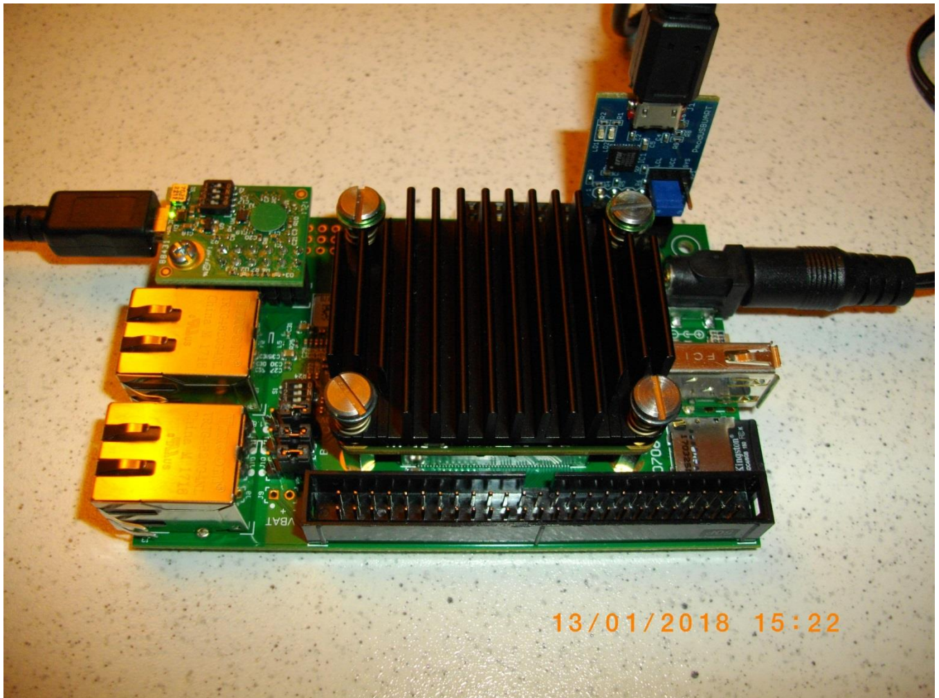
Figure 1: TE0706-02 carrier board with TE0720-2IF Zynq module
